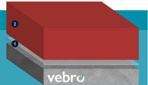
vebrocreed SBR can be installed and laid to falls prior to the installation of vebrocrete HF to ensure sufficient drainage.
