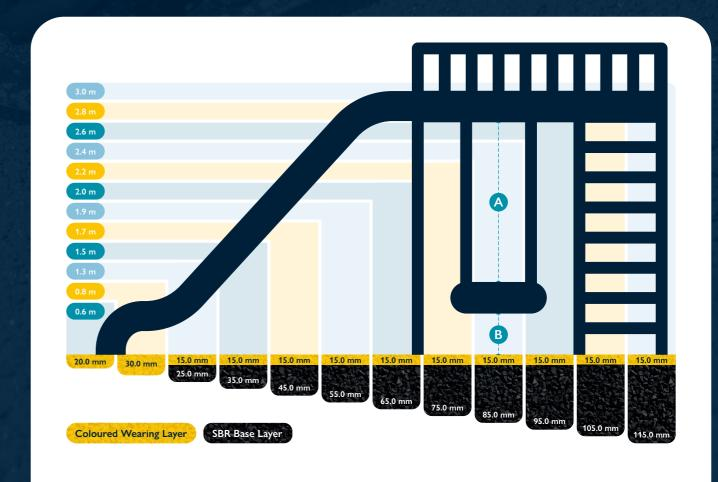
Swings are slightly different to stationary play equipment. The FFH for swings is measured from the centre of the stationary swing seat at 60 degrees.
