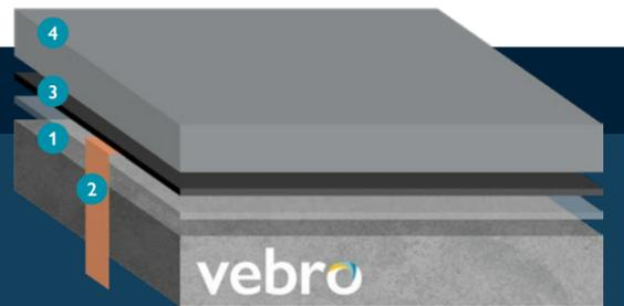
Enhanced slip resistance can be achieved with vebrostatic ESD SL SR (Conductive).
